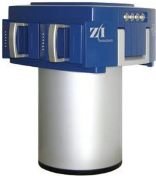
Figure 2 - (a) The Intergraph RMK D medium-format airborne digital camera showing the handles of two of the solid-state disk (SSD) units on its left side and one of its carrying handles on its right side. (b) The DALSA FT53 CCD frame-type image sensor that is used to record the 6k x 6.8k (= 42 Megapixels) images on each of the camera's four multi-spectral channels.
