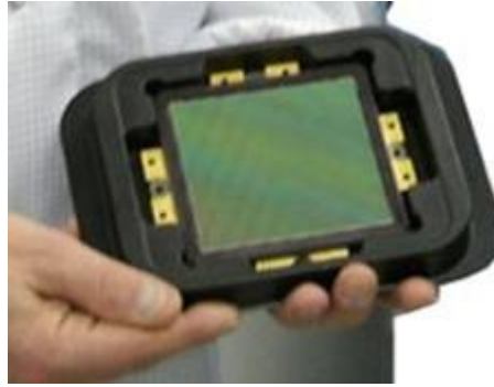
Figure 3 – The first 100+ Megapixel CCD imaging sensor that was built by DALSA SemiConductor in 2006 for use in an astronomical application by the U.S. Naval Observatory (USNO).
